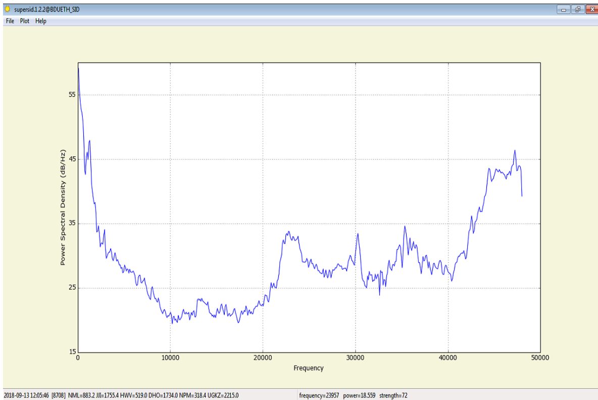
Figure 4.3: Interference affecting radio transmissions at receiver site
