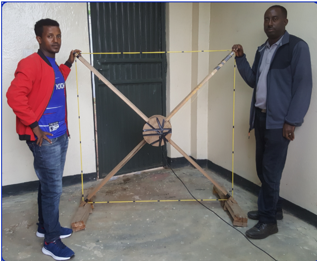
Figure 3.12: The large VLF antenna we constructed for our monitor: Picture, me with my thesis advisor Dr. Melessew Nigussie (Right).
