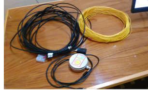
Figure 3.2: Antenna Wire (Yellow) and Coaxial Cable (Black).
