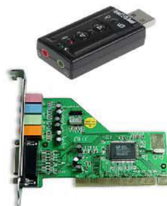
Figure 3.10: Sound cards to convert analog signals into digital , (Scherrer et al. , 2015)
