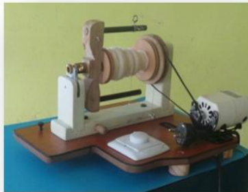
Figure3.20 fully assembled modified power driven spinning wheel with stand.
