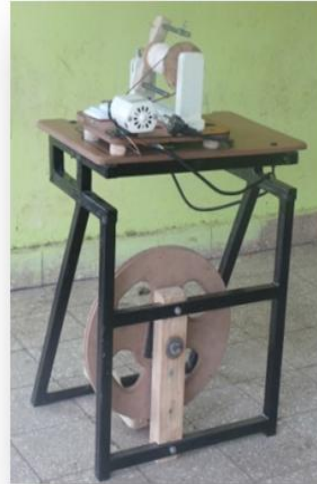
Figure3.20 fully assembled modified power driven spinning wheel with stand.
