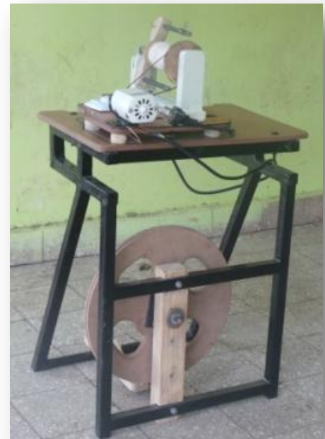
Picture while I am fabricating and producing parts, size and shape and assembling some parts of power driven spinning wheel in Gondar polytechnic college
