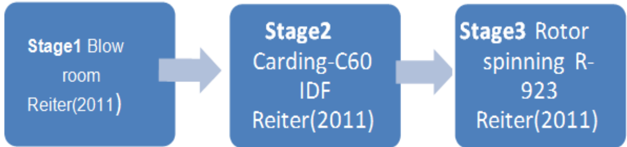
Figure.3.3 Cotton processing from blow room to rotor spinning
