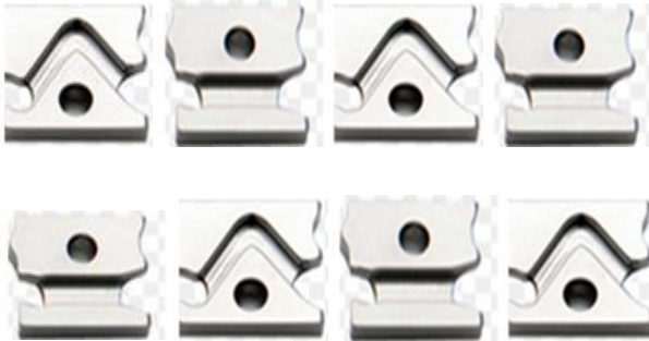
Figure 3 Cam and needle arrangement of cross miss structure
