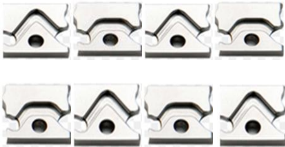
Figure 4 Cam and needle arrangement of single pique structure
