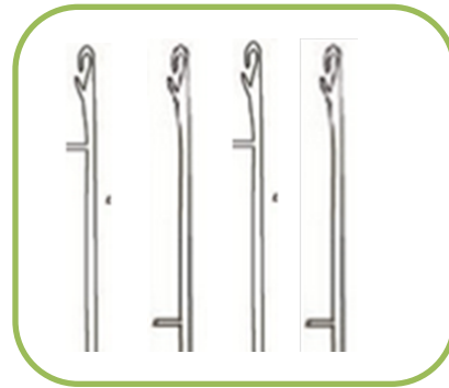
Figure 3 Cam and needle arrangement of cross miss structure
