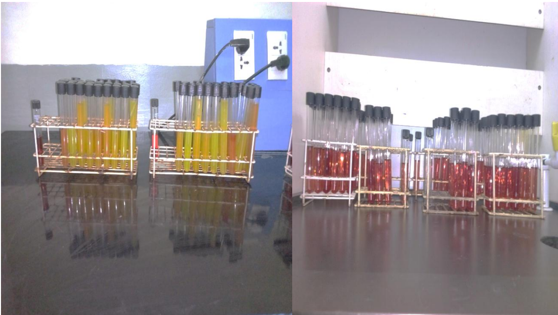
Media preparation and Presumptive Tests of indicator Microorganisms( fecal and total coliform)
