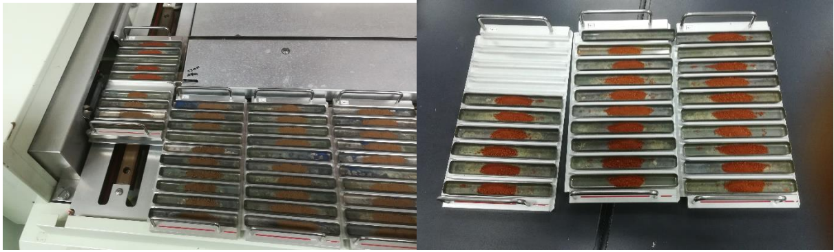
Appendix Figure 5.1 Determination of forage nitrogen and carbon level, samples injecting to CN coder machine (left) and after burning for extraction (right)
