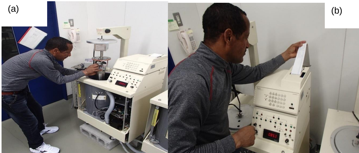
Appendix Figure 5.2 Determination of gross energy using bomb calorimeter, injecting in to bomb calorimeter (a) and data observation (b) in Shimane Science and Technology.
