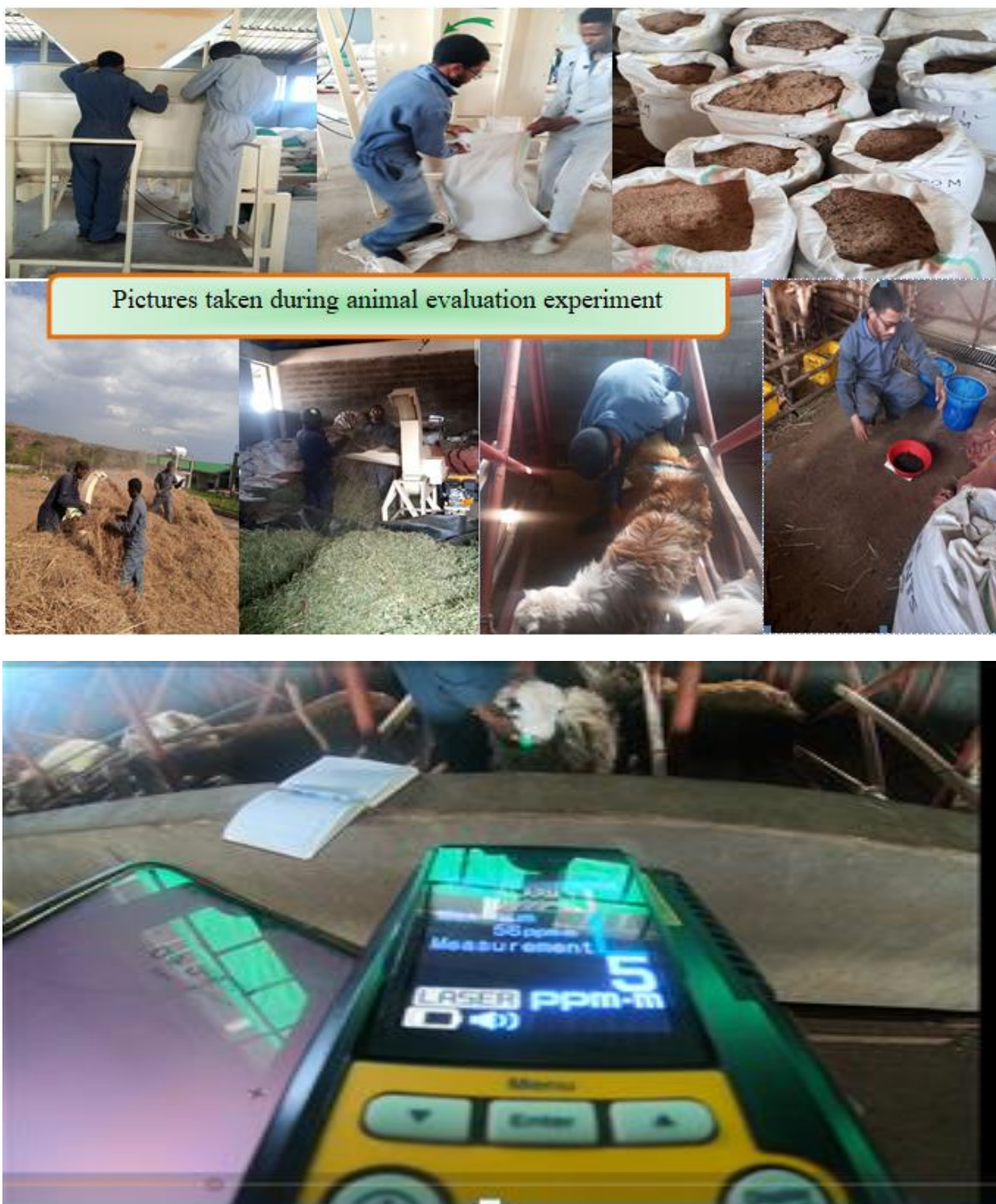
Figure 7.1. Methane emission measuring using laser methane detector (LMD) during the experiment
