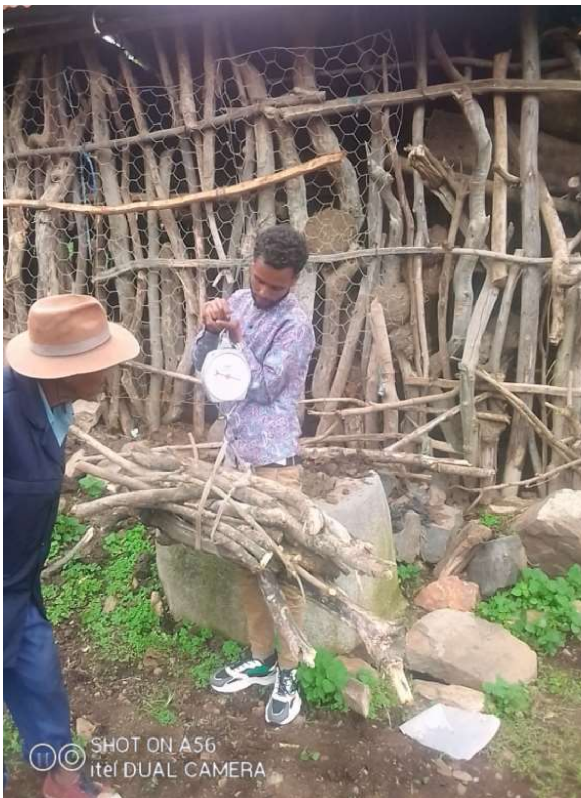
Figure 2: Photos taken during KPT measurements of fuel wood
