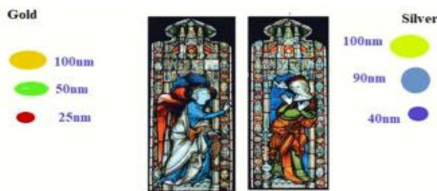
Figure 2.15: The colors of gold and silver nanomaterials are size-dependent, as are their effects on the coloring of stained glass. 142
