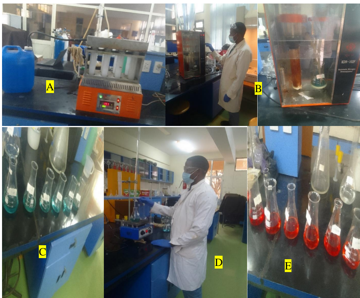
Figure 5.4. Determination of percent total nitrogen by the Kjeldahl method. A. Digestion. B. Distillation. C. Result of distillation. D. Titration. E. Pink colour after titration
