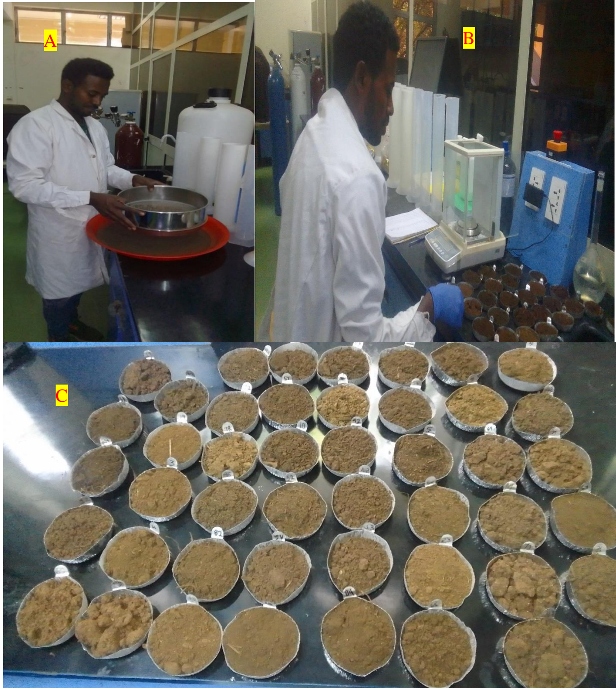
Figure 5.3. Physical properties of the soil sample in the laboratory (determining the bulk density). A. Soil sieving. B. Measuring the weight of oven-dried soil C. Result of oven-dried soil sample measured for bulk density
