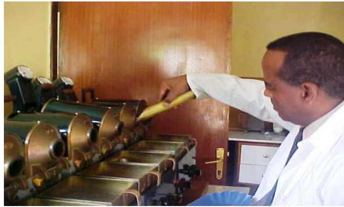
Figure 1: Samples Coffee roasting using a sample roaster machine (six-cylinder roaster).
