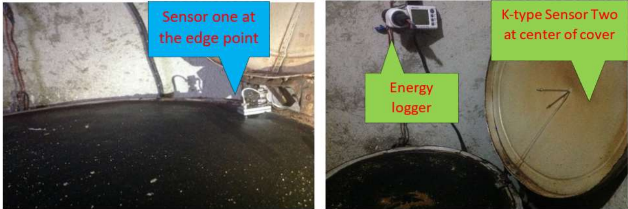
Figure 3.13. Experimental setup of K-type thermocouple sensors and energy logger on EIBM.
