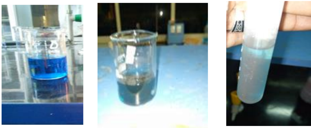
Figure 18: Photocatalytic degradation of MG dye using synthesized clay-supported CuO NCPs.
