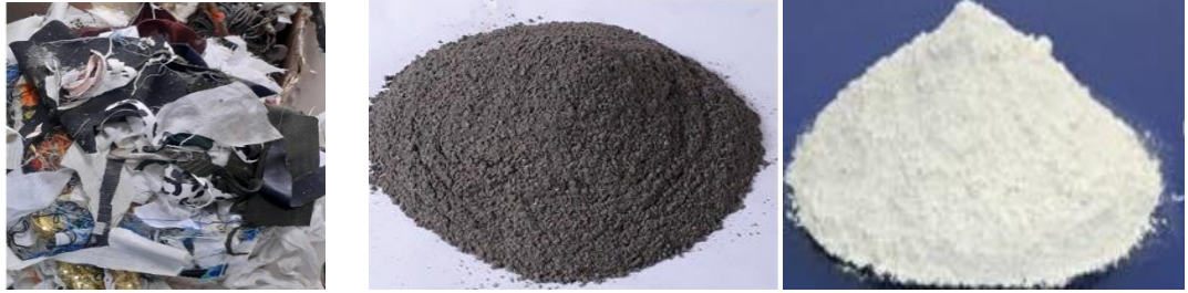
a) Synthetic cloth waste b) Synthetic cloth waste ash c) Lime
