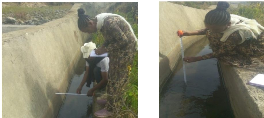
Figure 3-4 Measuring canal width and depth on the upper canal section (Source: Photo taken on December 22/2023 during field survey)
