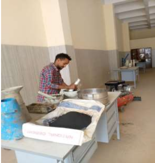
Figure 3.4 Grinding and sieving burned cattle bone
