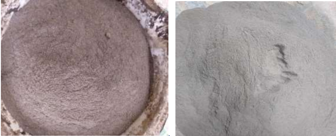
Figure 3.3. Sugarcane Bagasse Ash before and after calcination
