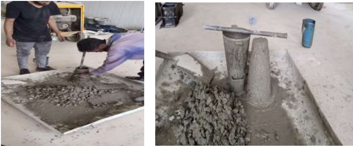
Figure 3.7 Sample slump test
