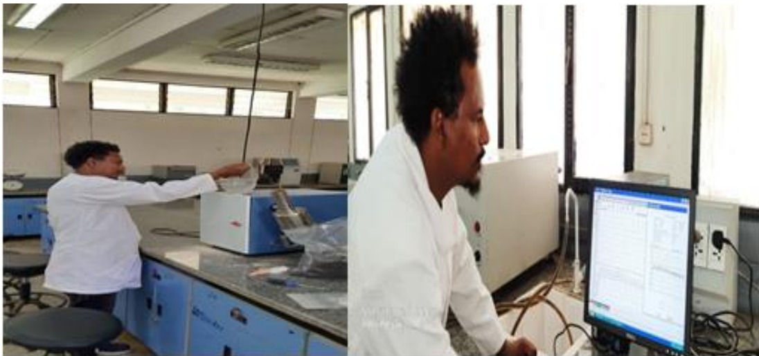
Working on laboratory miller for preparation of flour and Brabender Farinograph for evaluation of Rheological properties of composite flour (food research lab)
