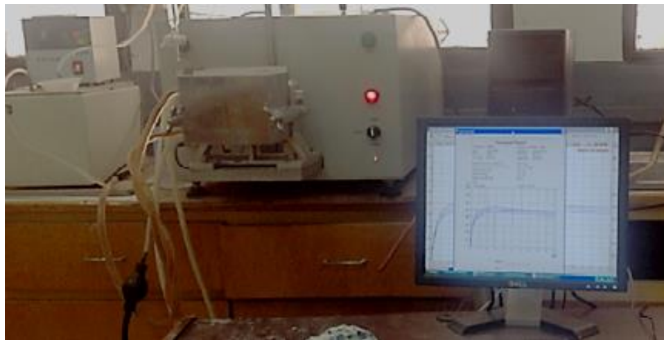
Figure 3. 1. An electronic farinograph used to measure physical dough properties
