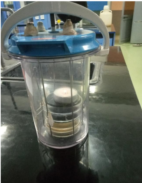
Plates with lighting candle in anaerobic jar
