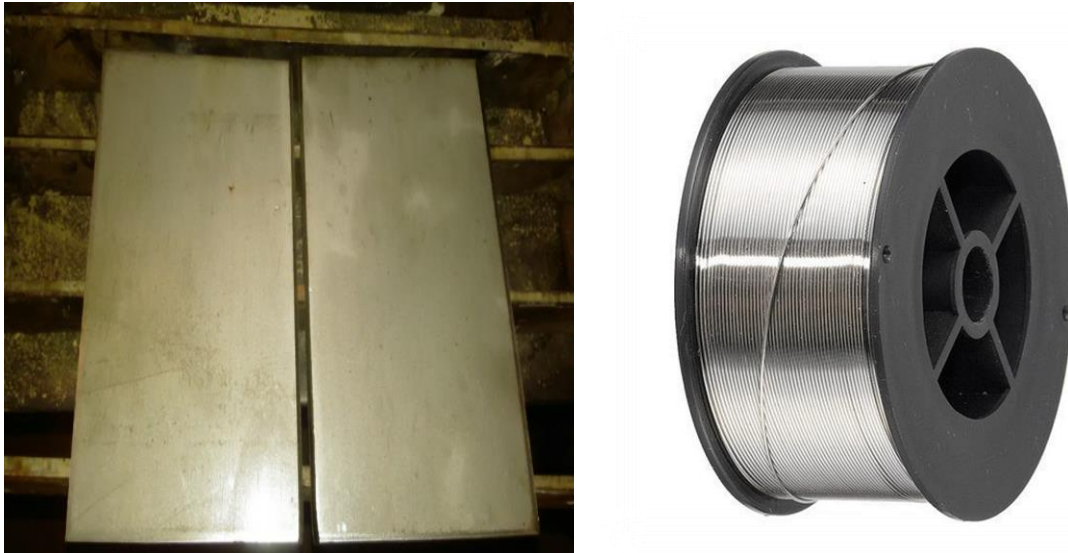
Figure 3.2. Specimen for welding SS304L and Wire Electrode SS308LSi
