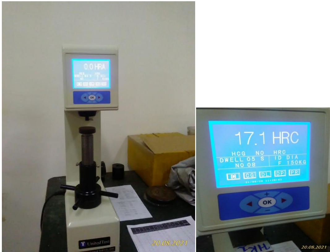
Figure 3.16. Rockwell Hardness Tester / Bench top / Digital Display
