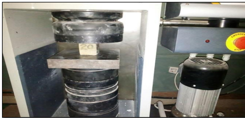
Figure 3-12: Compression Strength Machine Used (A) and Screen Display (B)
