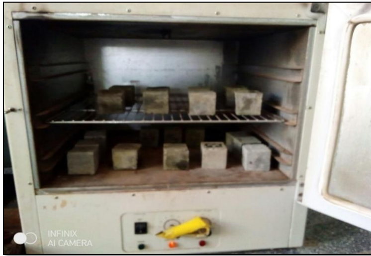
Figure 3-13: Specimen Oven Drying For Water Absorption
