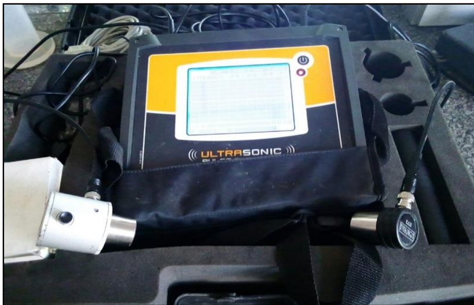
Figure 3-14: Ultrasonic Pulse Velocity Apparatus Used
