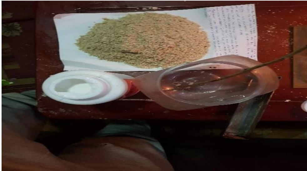
Fig 3.5 Mixing Maize Cob and urea formaldehyde
