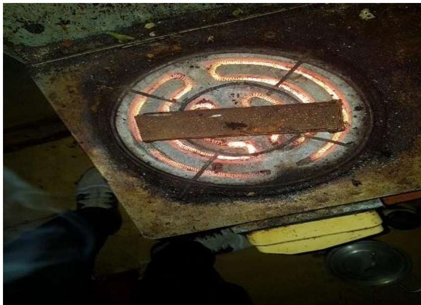
Fig 3.8 Stove for heating the specimen to the desired temperature
