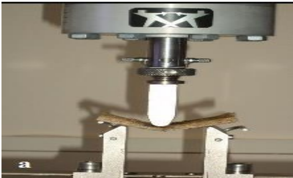
Figure 3.10 Universal testing machine for testing of flexural strength
