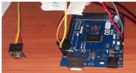
Figure 3.5: MLX90614 Temperature sensor with Arduino
