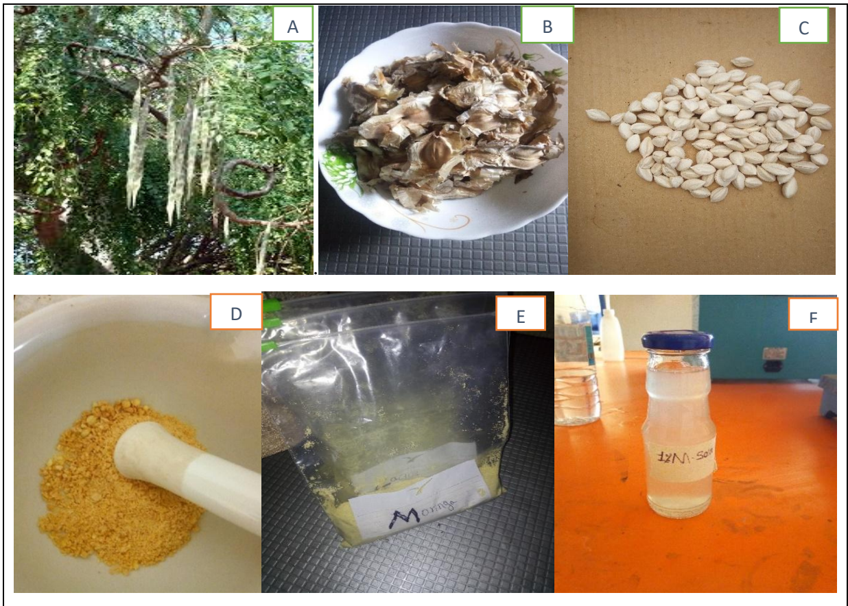
Figure 7:1 Bio-coagulant extraction process from moringa stenopetalla plant(A-F) (source from photo).
