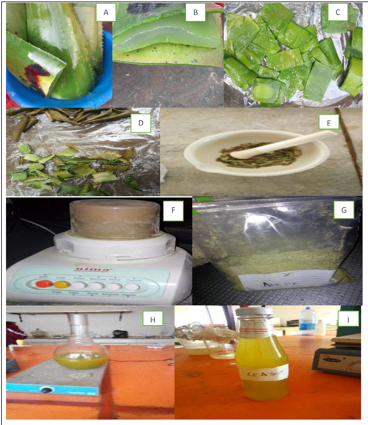
Figure 7:2 Bio-coagulant extraction process from Aloe Vera plant (A-I) (source from photo).
