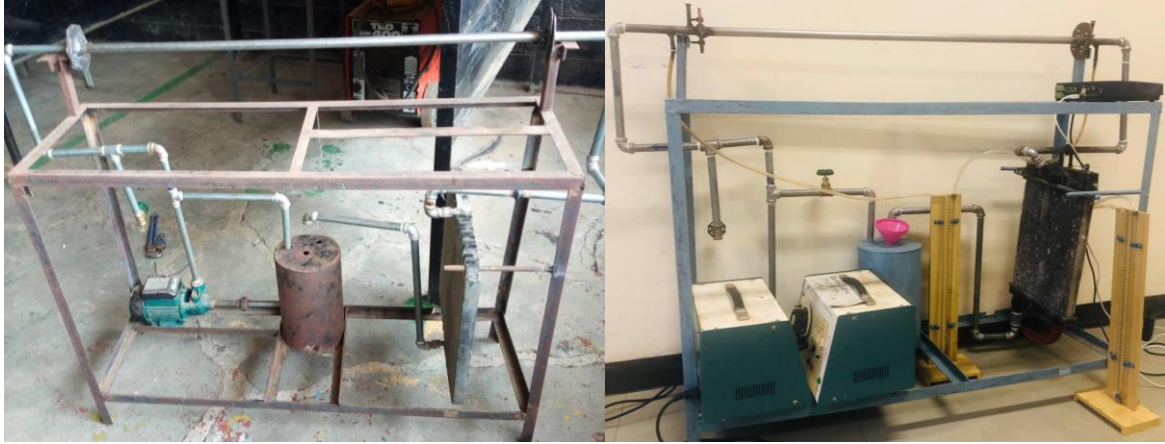
Figure 3-8 Flow loop with power supply reservoir, heat exchanger and manometers fixed A simple concentric orifice plate made from 30mm diameter thin stainless-steel sheet with a 12 mm round edged circular hole was fixed in the flow loop. A U-tube manometer was tapped one pipe diameter across the orifice plate (both upstream and downstream) to measure the pressure drop.
