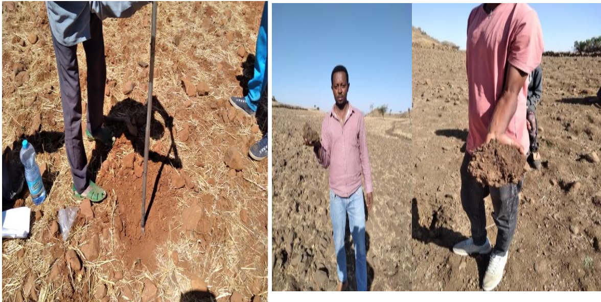
Appendix figure 2. Taking soil samples using auger and identifying soil structural class
