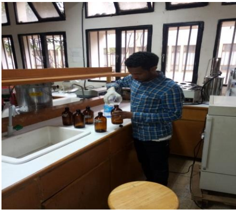
Water sample dropped into BOD bottle and after fifth days reading
