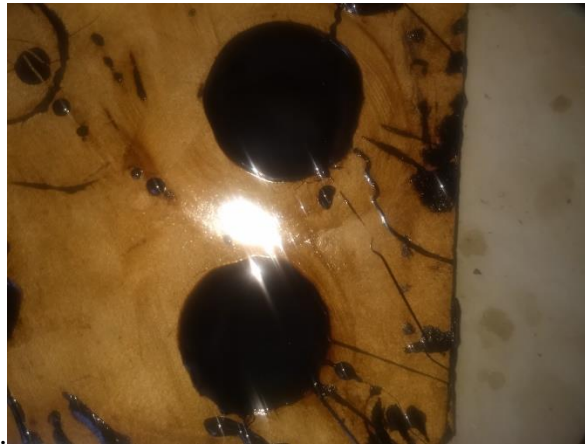
Figure 13: Prepared sample for DSR testing (25mm) plate
