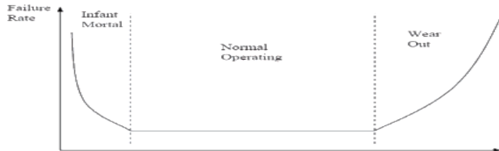
Figure3. 5: Bathtub curve of a component life
