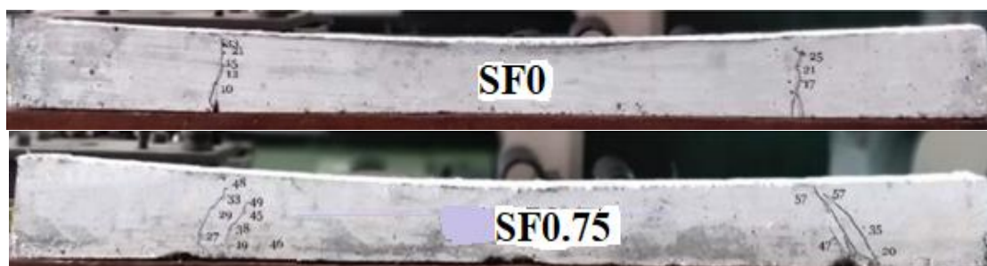
Figure 4. 2 Damage pattern on sleeper subjected to rail seat static test (Anand R. et al. 2020)
