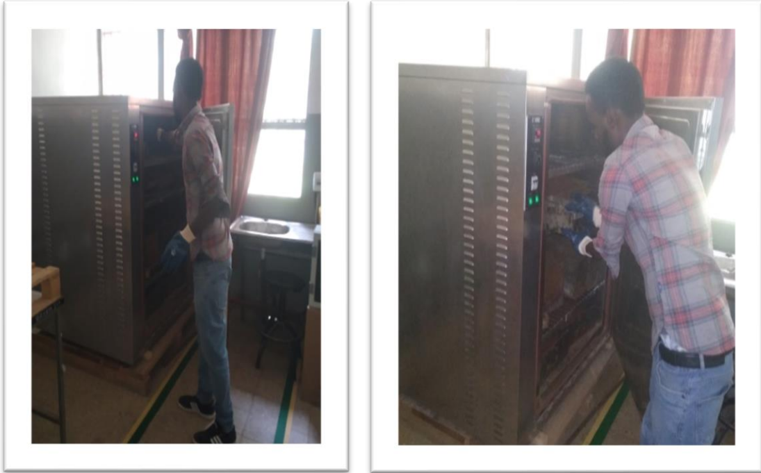
Figure C.3: Putting the sample (sand and steel slag) and cubes for water absorption in the oven
