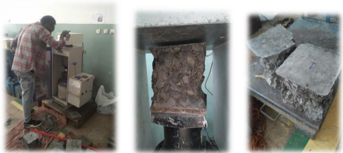
Figure 4. 2: Compressive strength test and failure Mechanism
