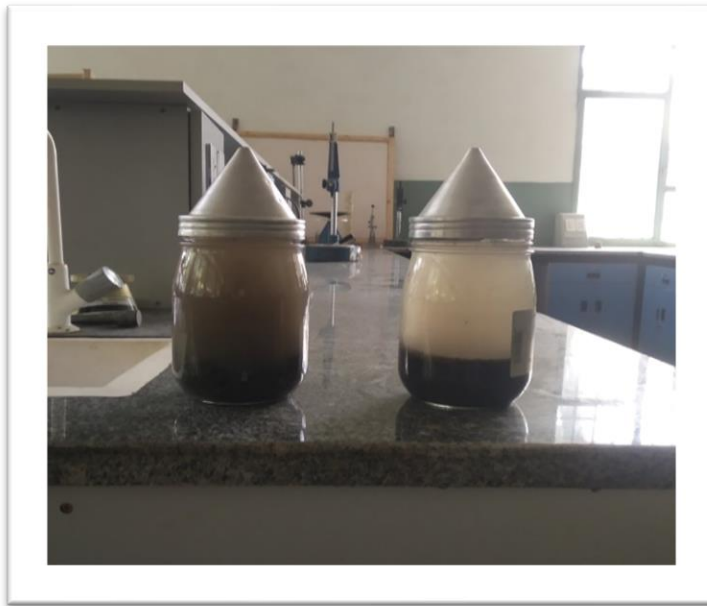
c) Natural sand and steel slag specific gravity test (sand @ the left and steel slag @ the right)
