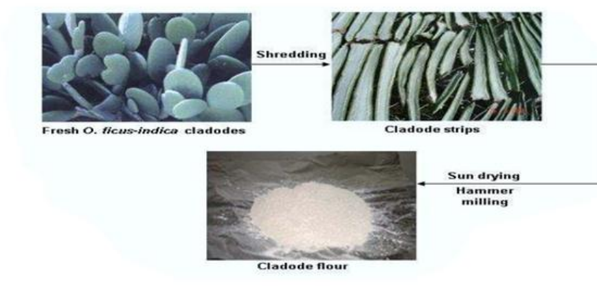
Figure3.2 Mechanical pretreatment of O. ficus-indica cladodes
