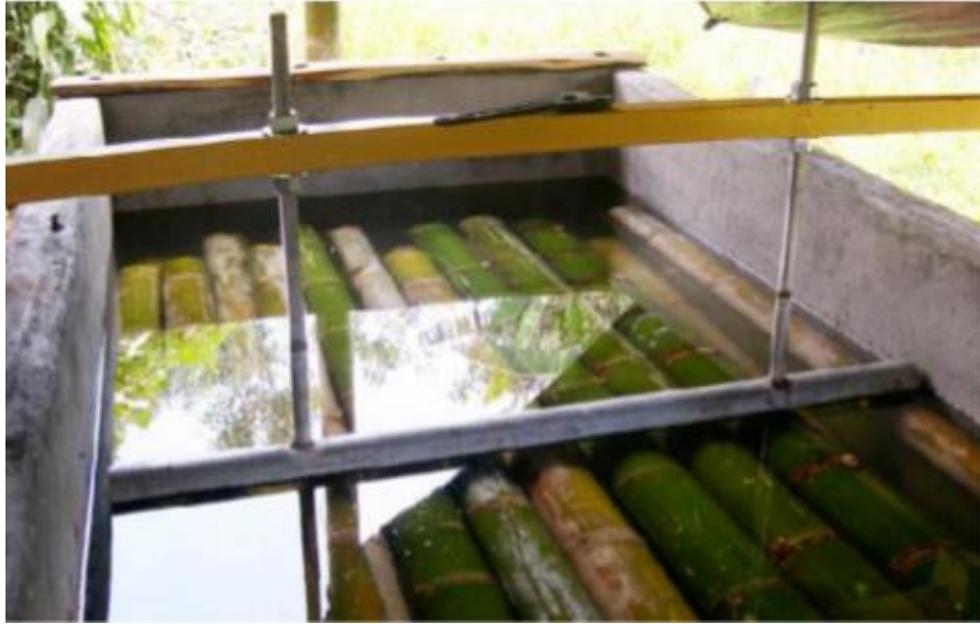
Figure 2. 11: Immersing bamboo in water [11]
