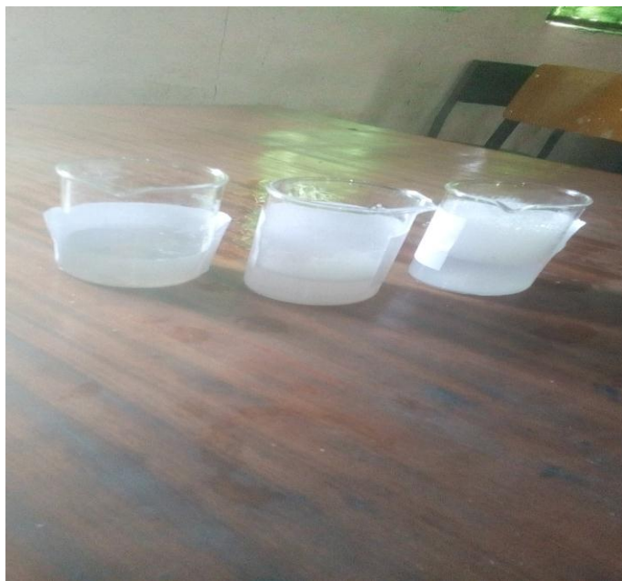
Figure 11 determination of hardness of water with soap
