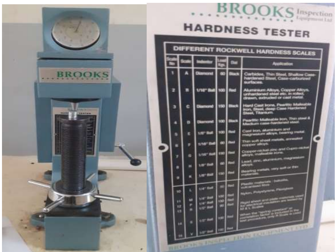
Figure 4.2 Rockwell hardness test machine and their scale.
