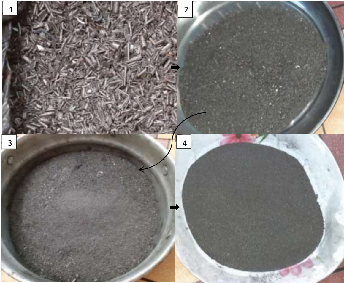
Figure 3.3 The size reduction of GGG-40 cast iron chips from 1 to 4.
