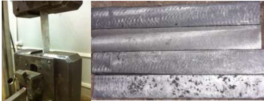
(a) Universal tensile testing machine (b) Tensile test specimen before test
