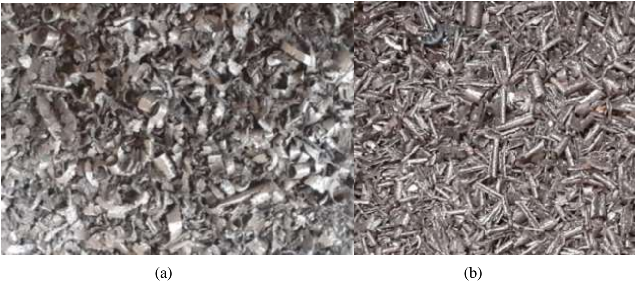
Figure 3.1 Used material: (a) AlMg1SiCu aluminum alloy chips, (b) GGG-40 cast iron chips.
