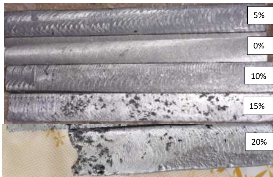
Figure 4.14 Using the prepared tensile test sample before test for microstructure examination
