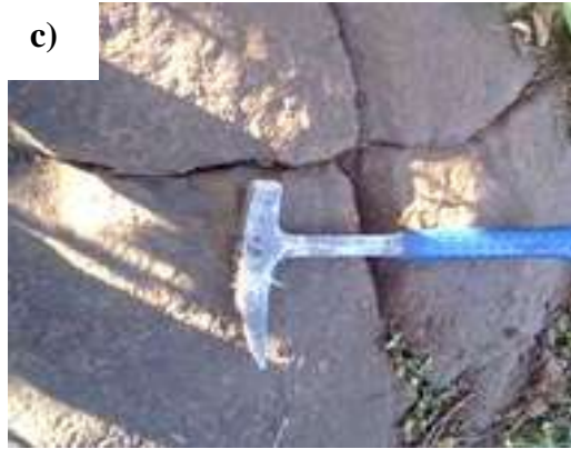
Figure 3.10) a joint on a basalt. A) Having a strike of N60W, dip amount of 50. B) Afield photograph showing columnar basalt exposed by Inbodbod river. C) X joint having a dip amount of 47 and a strike of S 22 E.
