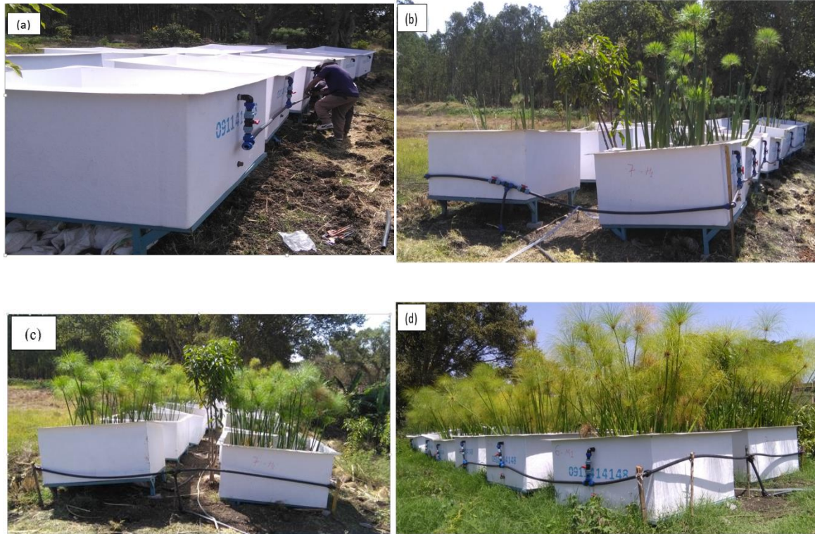
Figure 3.3 Installation (a), plantation day (b), after eight weeks (c) and after fourteen weeks (d) Aspect of C. papyrus in the glass fiber tanks constructed Wetlands.
