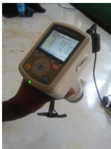
Figure 8: Spectrophotometer used for flour color measurement.
