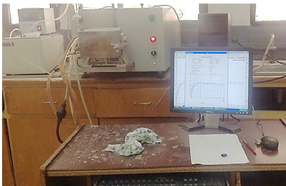
Figure 5: Farinograph instrument installed in the food safety laboratory, Institute of Technology, Bahir Dar University
