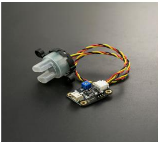
Figure 11: Water turbidity sensor device and specifications
