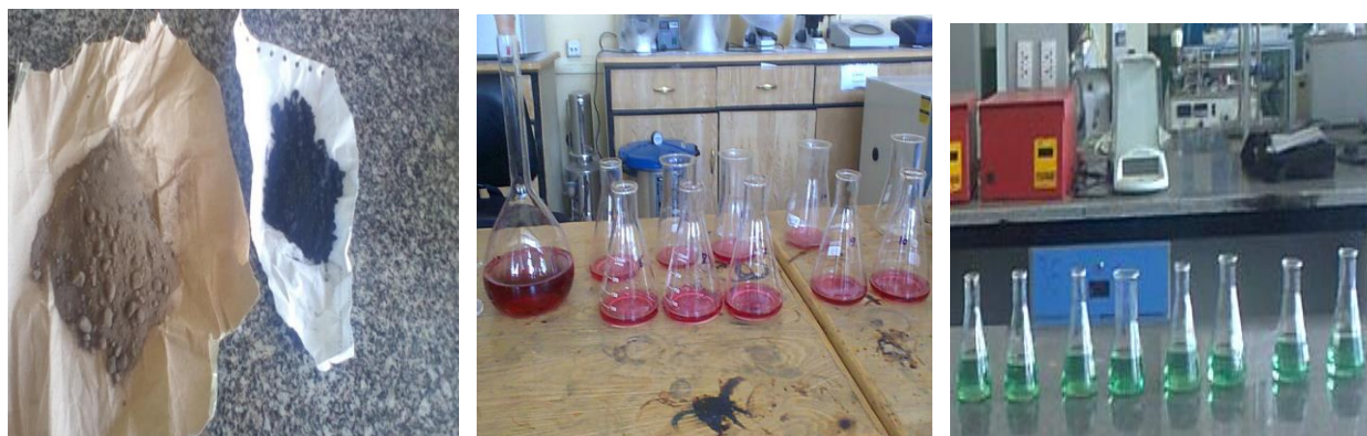
Weight compost after burning 1.4% boric acid solution with indicator After distillation to determine T-N
