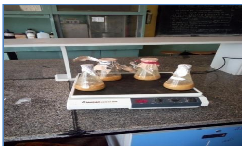
Figure 3.3. Orbital shaker solvent extraction
