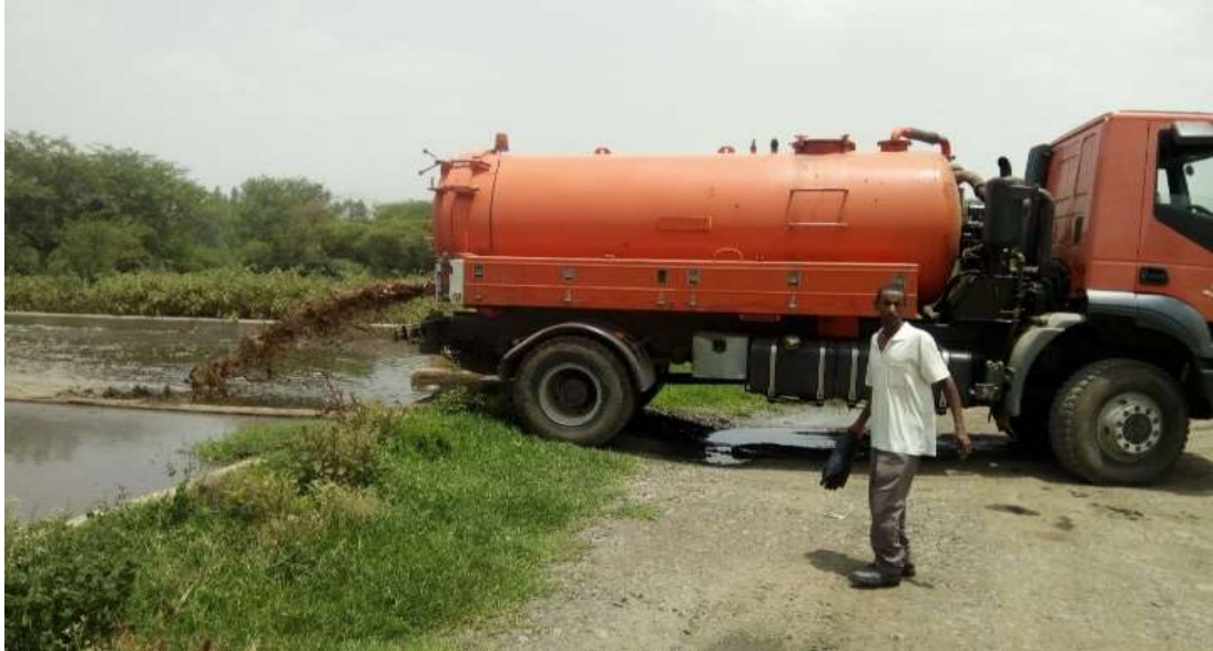
Figure 4.4a: Municipal vacuum truck discharging fecal sludge at FSTP
