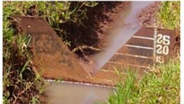
Graded V- Notch weir installed at QC
