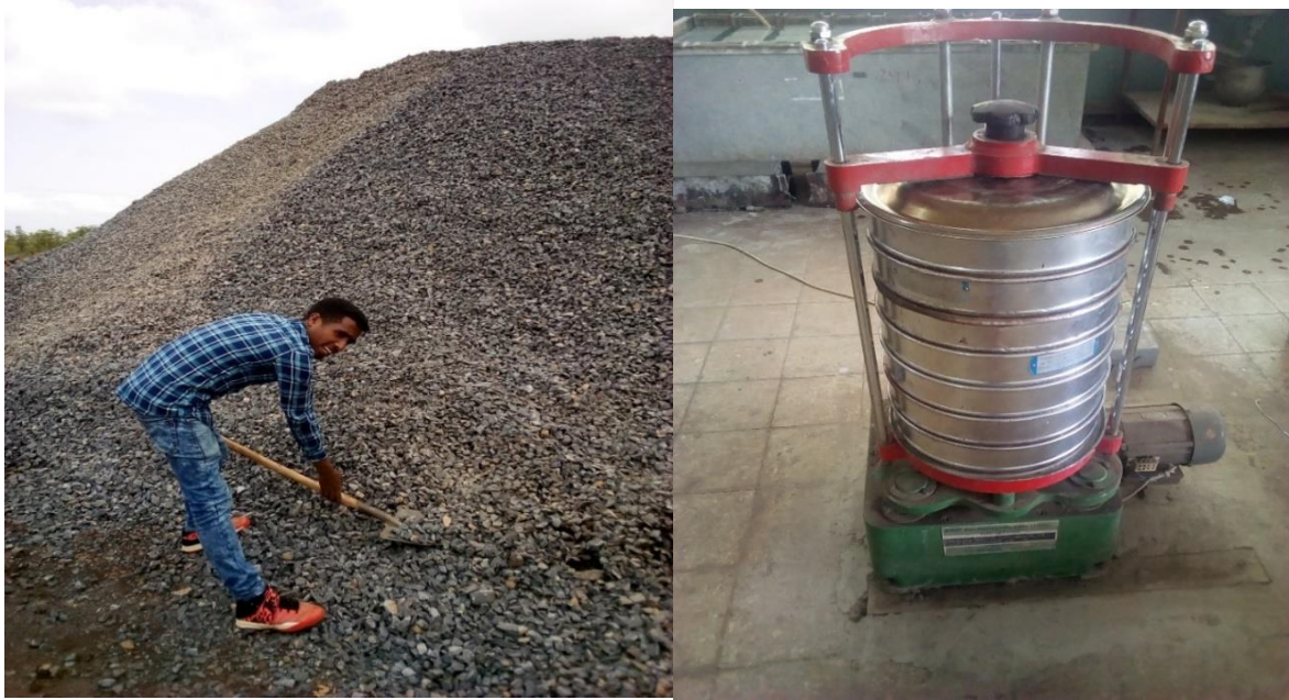
Figure 7-4: Aggregate Selection in Bahir Dar(left) & Aggregate gradation test (right)
