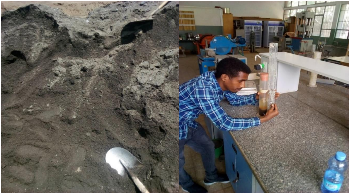
Figure 7-5: Selected Lalibela Sand in Bahir Dar (left) and Silt Content Test (right)
