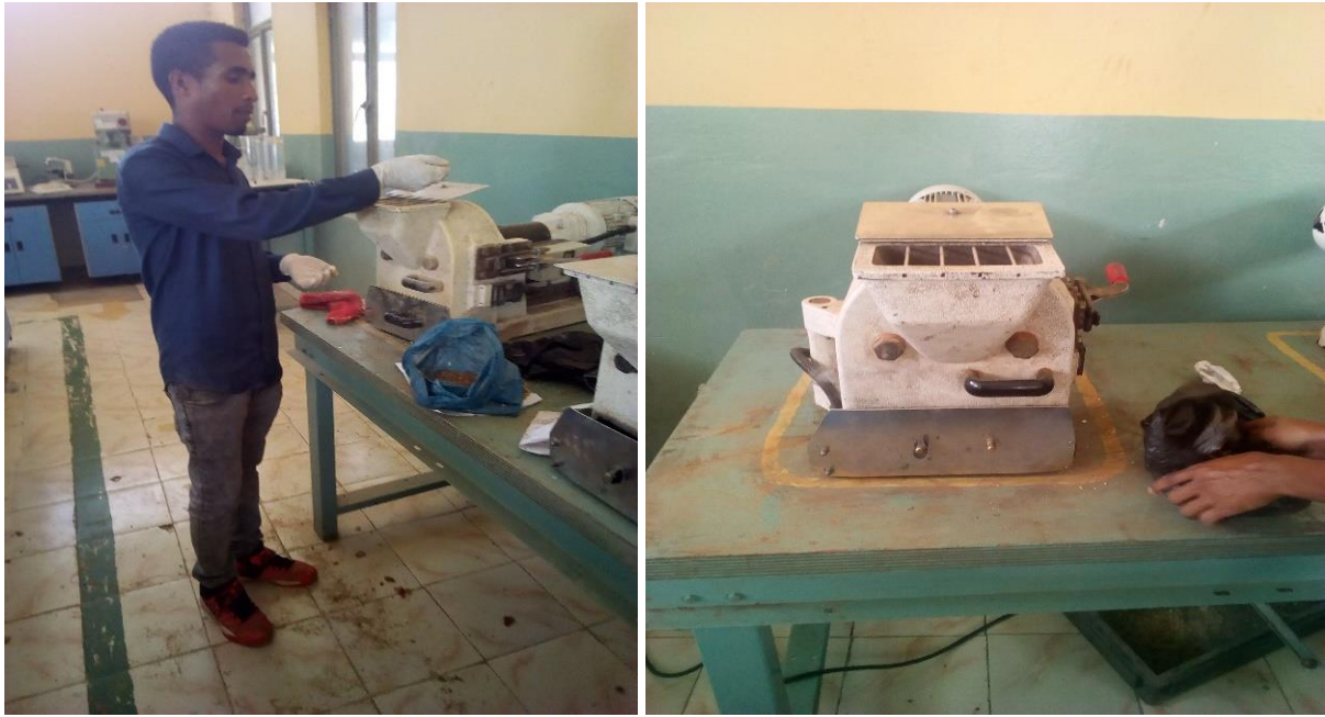
Figure 4-5: Bone Ash Milling by Disk Mill
