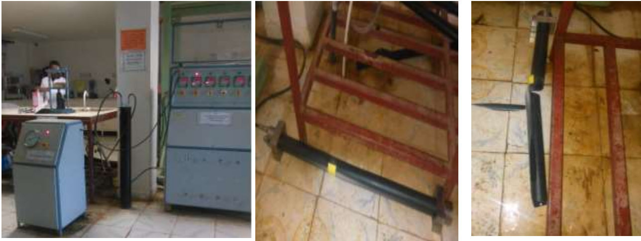
Hydrostatic pressure test machine pipes before and after bursting by hydrostatic pressure
