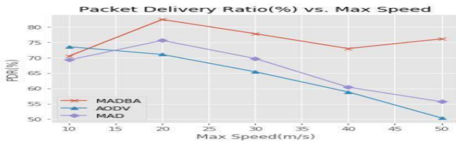
Figure 4. 6 Packet Delivery Ratio vs. Max Speed
