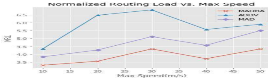
Figure 4. 9 Normalized Routing Load vs. Max Speed
