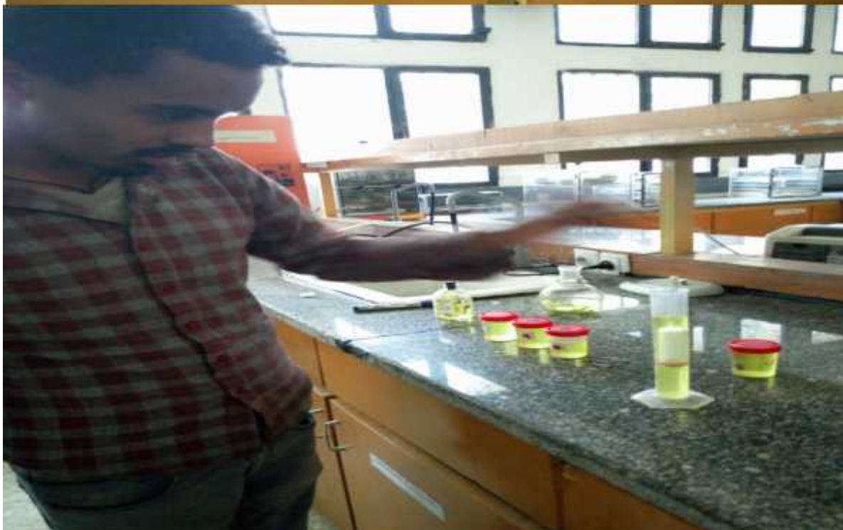
Figure I: Specific gravity measurement using a hydrometer
