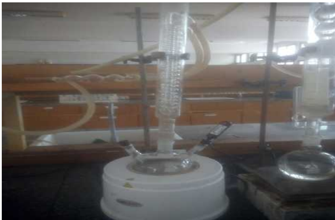
Figure C: Transesterification process laboratory set-up
