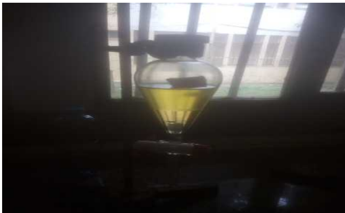
Figure D: separation of biodiesel and glycerol
