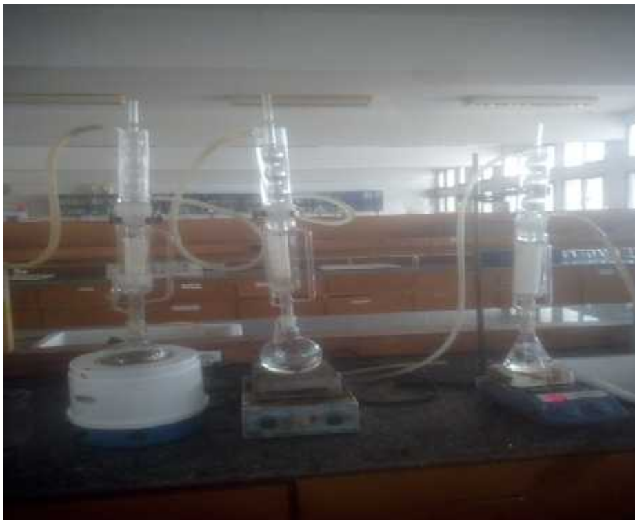
Figure 3.3 Soxhlet extraction setup
