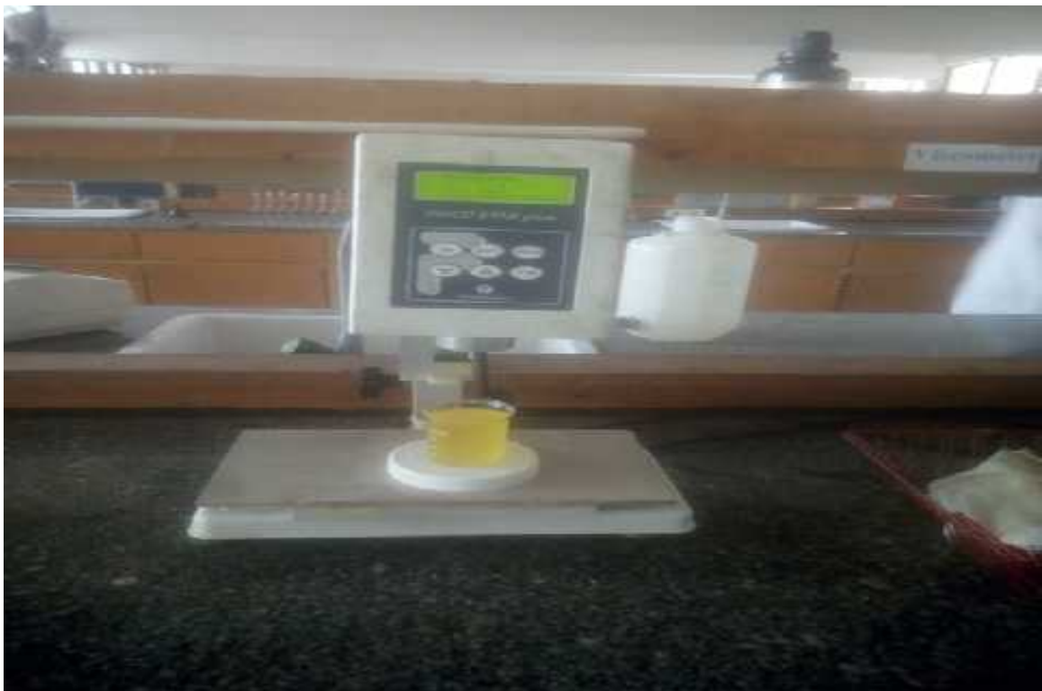
Figure F: Viscosity measurement using viscometer
