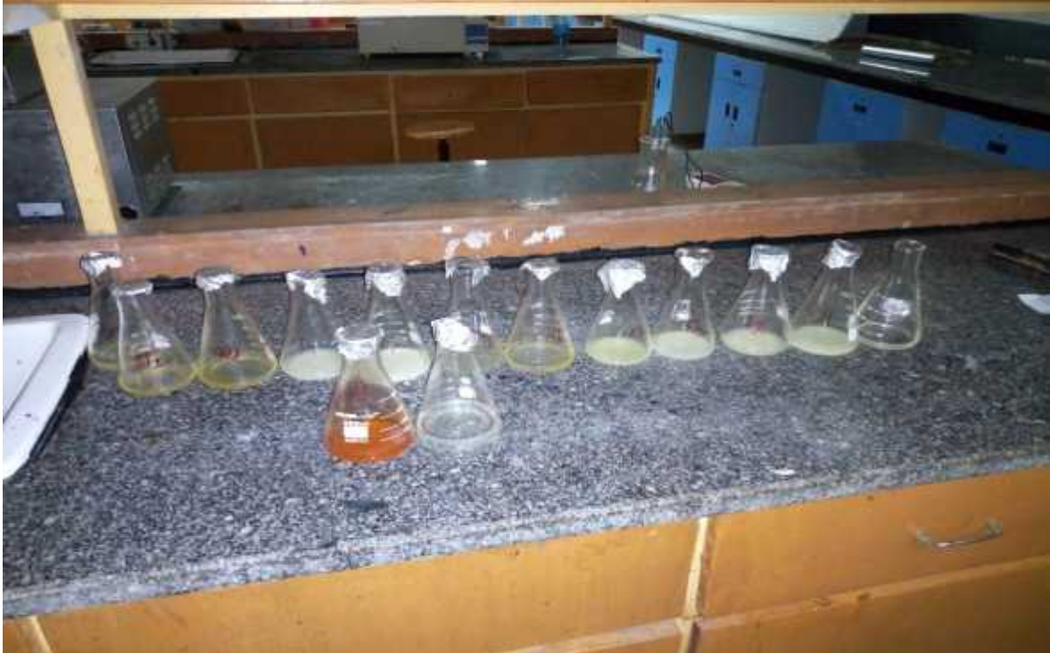
Figure H: Saponification value determination using titration
