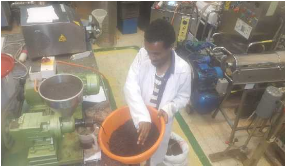
Figure A: Oil extraction using mechanical press machine
