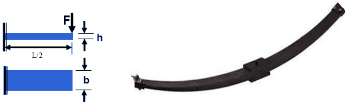
Figure 3.1: Important dimensions and free body diagram to analyze half of the leaf spring [29]
