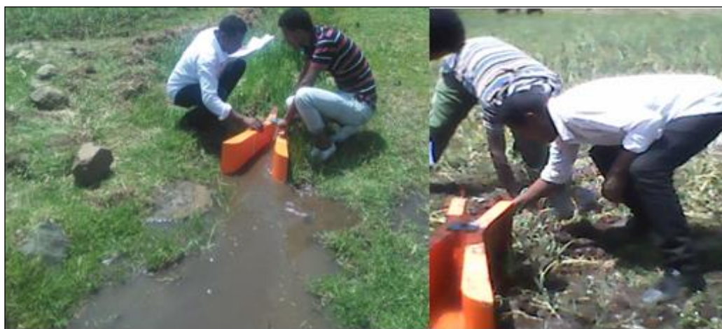
Figure 4.1 Discharge measurement using 3 inch Parshall flume
