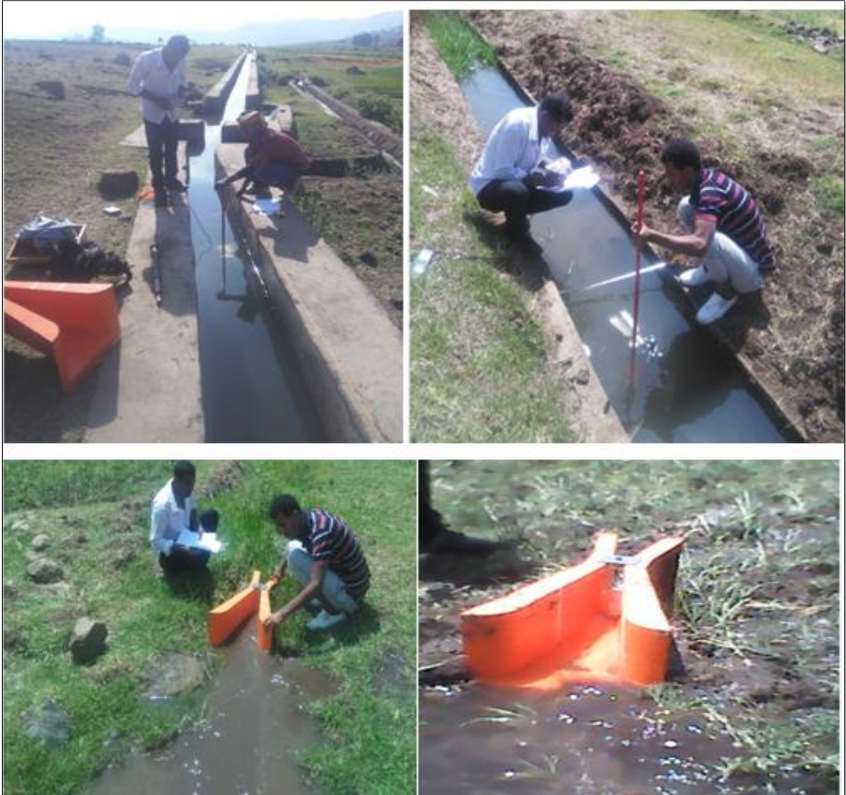
Figure 3.7: Discharge Measurement Using Current Meter and Parshall Flumes
