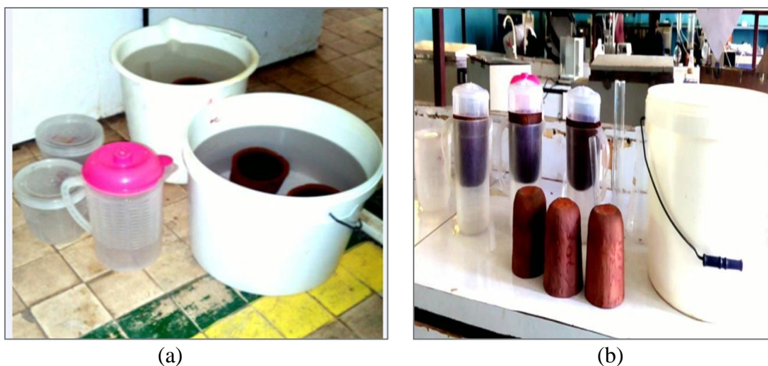
Figure 3.7 Ceramic water filters soaking in water and Quantity of water filtered testing
