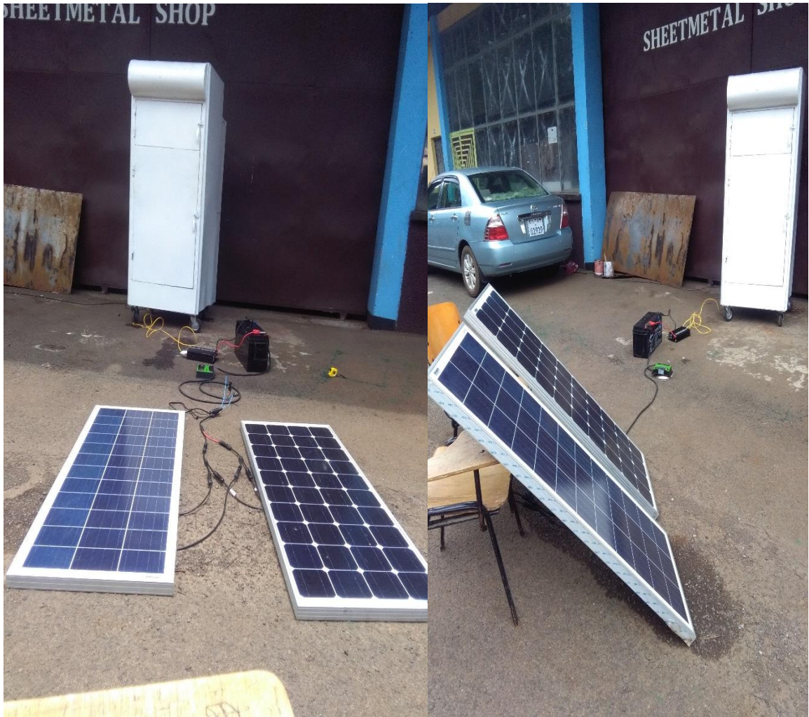
Figure 4. 1: Pictures of experimental test set up of evaporative cooling.
