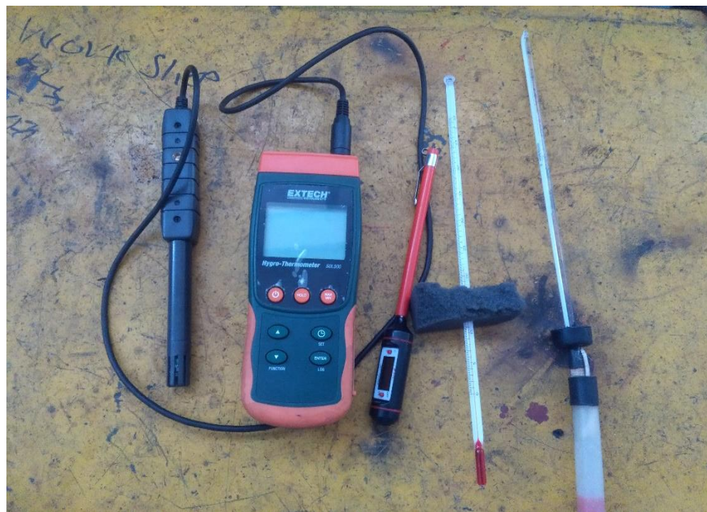
Figure 4. 3: Temperature and relative humidity measuring devices.
